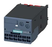
electronic timing relay, off delayed, with control signal and semiconductor output, time range 0.05-100 s, 24-90 V AC/DC, 50/60 Hz, varistor for attenuation of the contactor coils integrated, spring-loaded terminal, can be snapped on at the front on contactors 3RT2.3 / 3RT2.4
