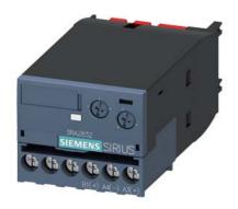
electronic timing relay, off delayed, with control signal and semiconductor output, time range 0.05-100 s, 90-240 V AC/DC, 50/60 Hz, varistor for attenuation of the contactor coils integrated, screw terminal, can be snapped on at the front on contactors 3RT2.3 / 3RT2.4
