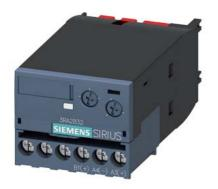
electronic timing relay, off delayed, with control signal and semiconductor output, time range 0.05-100 s, 24-90 V AC/DC, 50/60 Hz, varistor for attenuation of the contactor coils integrated, screw terminal, can be snapped on at the front on contactors 3RT2.3 / 3RT2.4
