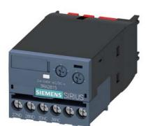
solid-state time-delayed auxiliary switch, off delayed, without control signal, relay 1 NC + 1 NO, time range 0.05-100 s, 24-240 V AC/DC, 50/60 Hz, varistor for attenuation of the contactor coils integrated, screw terminal, can be snapped on at the front on contactors 3RT2 and auxiliary contactors 3RH2
