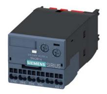
solid-state time-delayed auxiliary switch, off delayed, with control signal, relay 1 NC  $\pm$  1 NO, time range 0.05-100 s, 24-240 V AC/DC, 50/60 Hz, varistor for attenuation of the contactor coils integrated, spring-loaded terminal, can be snapped on at the front on contactors 3RT2 and auxiliary contactors 3RH2
