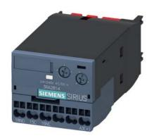
solid-state time-delayed auxiliary switch, off delayed, with control signal, relay: 1 CO, time range 0.05-100 s, 24-240 V AC/DC, 50/60 Hz, varistor for attenuation of the contactor coils integrated, spring-loaded terminal, can be snapped on at the front on contactors 3RT2 and auxiliary contactors 3RH2
