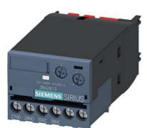
solid-state time-delayed auxiliary switch, ON-delay, relay 1 NC + 1 NO, time range 0.05-100 s, 24-240 V AC/DC, 50/60 Hz, varistor for attenuation of the contactor coils integrated, screw terminal, can be snapped on at the front on contactors 3RT2 and auxiliary contactors 3RH2
