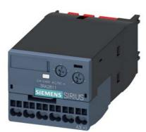
electronic timing relay, ON-delay, with semiconductor output, time range 0.05-100 s, 24-240 V AC/DC, 50/60 Hz, varistor for attenuation of the contactor coils integrated, spring-loaded terminal, can be snapped on at the front on contactors 3RT2.1 / 3RT2.2 and auxiliary contactors 3RH2
