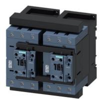
reversing contactor assembly, AC-3e/AC-3, 110 A, 55 kW / 400 V, 3-pole, 20-33 V AC/DC, 50/60 Hz, screw terminal, electrical and mechanical interlock, auxiliary contacts: 2 x 1 NO, with voltage tap for 3RA27
