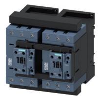
reversing contactor assembly, AC-3e/AC-3, 95 A, 45 kW / 400 V, 3-pole, 20-33 V AC/DC, 50/60 Hz, screw terminal, electrical and mechanical interlock, auxiliary contacts: 2 x 1 NO
