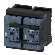
reversing contactor assembly, AC-3e/AC-3, 95 A, 45 kW / 400 V, 3-pole, 230 V AC, 50/60 Hz, screw terminal, electrical and mechanical interlock, auxiliary contacts: 2  $\times$  1 NO
