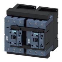
reversing contactor assembly, AC-3e/AC-3, 95 A, 45 kW / 400 V, 3-pole, 110 V AC, 50/60 Hz, screw terminal, electrical and mechanical interlock, auxiliary contacts: 2 x 1 NO
