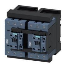
reversing contactor assembly, AC-3e/AC-3, 80 A, 37 kW / 400 V, 3-pole, 20-33 V AC/DC, 50/60 Hz, screw terminal, electrical and mechanical interlock, auxiliary contacts: 2 x 1 NO, with voltage tap for 3RA27
