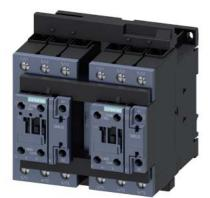
reversing contactor assembly, AC-3e/AC-3, 80 A, 37 kW / 400 V, 3-pole, 20-33 V AC/DC, 50/60 Hz, screw terminal, electrical and mechanical interlock, auxiliary contacts: 2 x 1 NO, with voltage tap for 3RA27
