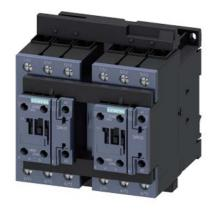
reversing contactor assembly, AC-3e/AC-3, 80 A, 37 kW / 400 V, 3-pole, 110 V AC, 50 Hz / 120 V, 60 Hz, screw terminal, electrical and mechanical interlock, auxiliary contacts: 2 x 1 NO
