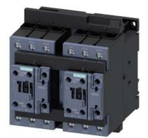
reversing contactor assembly, AC-3e/AC-3, 80 A, 37 kW / 400 V, 3-pole, 110 V AC, 50/60 Hz, screw terminal, electrical and mechanical interlock, auxiliary contacts: 2 x 1 NO
