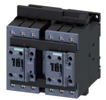
reversing contactor assembly, AC-3e/AC-3, 65 A, 30 kW / 400 V, 3-pole, 20-33 V AC/DC, 50/60 Hz, screw terminal, electrical and mechanical interlock, auxiliary contacts: 2 x 1 NO
