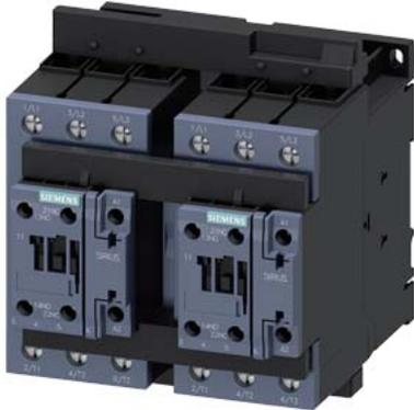
reversing contactor assembly, AC-3e/AC-3, 65 A, 30 kW / 400 V, 3-pole, 24 V DC, 0.7-1.25\* Us, with varistor plugged on, screw terminal, electrical and mechanical interlock, auxiliary contacts: 2 x 1 NO
