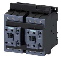
reversing contactor assembly, AC-3e/AC-3, 65 A, 30 kW / 400 V, 3-pole, 220 V AC, 50 Hz / 240 V, 60 Hz, screw terminal, electrical and mechanical interlock, auxiliary contacts: 2 x 1 NO
