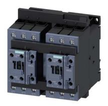
reversing contactor assembly, AC-3e/AC-3, 51 A, 22 kW / 400 V, 3-pole, 24 V DC, 0.7-1.25\* Us, with varistor plugged on, screw terminal, electrical and mechanical interlock, auxiliary contacts: 2 x 1 NO
