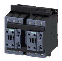
reversing contactor assembly, AC-3e/AC-3, 51 A, 22 kW / 400 V, 3-pole, 230 V AC, 50/60 Hz, screw terminal, electrical and mechanical interlock, auxiliary contacts: 2 x 1 NO
