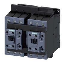
reversing contactor assembly, AC-3e/AC-3, 41 A, 18.5 kW / 400 V, 3-pole, 20-33 V AC/DC, 50/60 Hz, screw terminal, electrical and mechanical interlock, auxiliary contacts: 2 x 1 NO, with voltage tap for 3RA27
