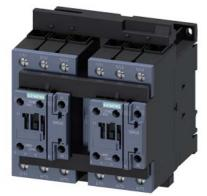
reversing contactor assembly, AC-3e/AC-3, 41 A, 18.5 kW / 400 V, 3-pole, 220 V AC, 50 Hz / 240 V, 60 Hz, screw terminal, electrical and mechanical interlock, auxiliary contacts: 2 x 1 NO
