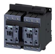
reversing contactor assembly, AC-3e/AC-3, 41 A, 18.5 kW / 400 V, 3-pole, 110 V AC, 50 Hz / 120 V, 60 Hz, screw terminal, electrical and mechanical interlock, auxiliary contacts: 2 x 1 NO
