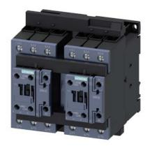
reversing contactor assembly, AC-3e/AC-3, 41 A, 18.5 kW / 400 V, 3-pole, 110 V AC, 50/60 Hz, screw terminal, electrical and mechanical interlock, auxiliary contacts:  $2\times1$  NO
