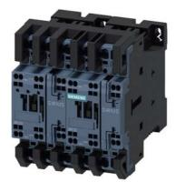
reversing contactor assembly, AC-3e/AC-3, 38 A, 18.5 kW / 400 V, 3-pole, 24 V DC, spring-loaded terminal, electrical and mechanical interlock, auxiliary contacts:  $2 \times 1$  NO, with voltage tap for 3RA27
