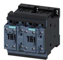
reversing contactor assembly, AC-3e/AC-3, 38 A, 18.5 kW / 400 V, 3-pole, 24 V DC, screw terminal, electrical and mechanical interlock, auxiliary contacts: 2 x 1 NO, with voltage tap for 3RA27
