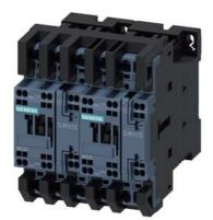
reversing contactor assembly, AC-3e/AC-3, 38 A, 18.5 kW / 400 V, 3-pole, 24 V DC, spring-loaded terminal, electrical and mechanical interlock, auxiliary contacts:  $2 \times 1 \text{ NO}$
