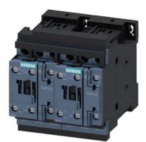
reversing contactor assembly, AC-3e/AC-3, 38 A, 18.5 kW / 400 V, 3-pole, 24 V DC, screw terminal, electrical and mechanical interlock, auxiliary contacts:  $2 \times 1$  NO
