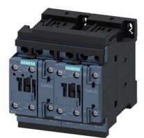
reversing contactor assembly, AC-3e/AC-3, 32 A, 15 kW / 400 V, 3-pole, 24 V DC, screw terminal, electrical and mechanical interlock, auxiliary contacts: 2 x 1 NO, with voltage tap for 3RA27
