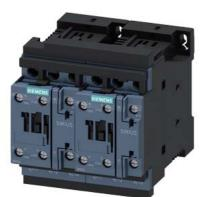
reversing contactor assembly, AC-3e/AC-3, 32 A, 15 kW / 400 V, 3-pole, 24 V DC, screw terminal, electrical and mechanical interlock, auxiliary contacts:  $2 \times 1 \text{ NO}$
