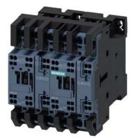
reversing contactor assembly, AC-3e/AC-3, 25 A, 11 kW / 400 V, 3-pole, 24 V DC, spring-loaded terminal, electrical and mechanical interlock, auxiliary contacts:  $2 \times 1$  NO, with voltage tap for 3RA27
