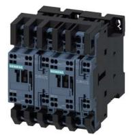
reversing contactor assembly, AC-3e/AC-3, 25 A, 11 kW / 400 V, 3-pole, 24 V DC, spring-loaded terminal, electrical and mechanical interlock, auxiliary contacts:  $2 \times 1$  NO
