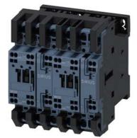
reversing contactor assembly, AC-3e/AC-3, 25 A, 11 kW / 400 V, 3-pole, 110 V AC, 50 Hz / 120 V, 60 Hz, spring-loaded terminal, electrical and mechanical interlock, auxiliary contacts:  $2 \times 1 \text{ NO}$
