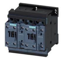
reversing contactor assembly, AC-3e/AC-3, 25 A, 11 kW / 400 V, 3-pole, 230 V AC, 50/60 Hz, screw terminal, electrical and mechanical interlock, auxiliary contacts: 2 x 1 NO
