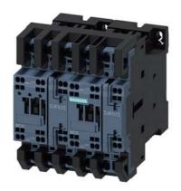
reversing contactor assembly, AC-3e/AC-3, 17 A, 7.5 kW / 400 V, 3-pole, 24 V DC, spring-loaded terminal, electrical and mechanical interlock, auxiliary contacts: 2 x 1 NO, with voltage tap for 3RA27
