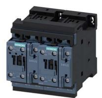
reversing contactor assembly, AC-3e/AC-3, 17 A, 7.5 kW / 400 V, 3-pole, 24 V DC, screw terminal, electrical and mechanical interlock, auxiliary contacts:  $2 \times 1 \text{ NO}$ , with voltage tap for 3RA27
