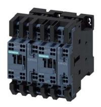
reversing contactor assembly, AC-3e/AC-3, 17 A, 7.5 kW / 400 V, 3-pole, 24 V DC, spring-loaded terminal, electrical and mechanical interlock, auxiliary contacts:  $2\times1$  NO
