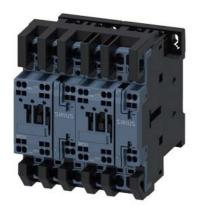
reversing contactor assembly, AC-3e/AC-3, 17 A, 7.5 kW / 400 V, 3-pole, 24 V AC, 50/60 Hz, spring-loaded terminal, electrical and mechanical interlock, auxiliary contacts: 2 x 1 NO
