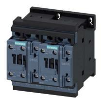
reversing contactor assembly, AC-3e/AC-3, 17 A, 7.5 kW / 400 V, 3-pole, 24 V AC, 50/60 Hz, screw terminal, electrical and mechanical interlock, auxiliary contacts: 2 x 1 NO
