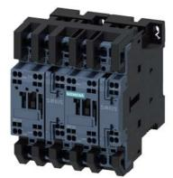
reversing contactor assembly, AC-3e/AC-3, 12 A, 5.5 kW / 400 V, 3-pole, 24 V DC, spring-loaded terminal, electrical and mechanical interlock, auxiliary contacts: 2 x 1 NO, with voltage tap for 3RA27
