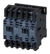
reversing contactor assembly, AC-3e/AC-3, 12 A, 5.5 kW / 400 V, 3-pole, 230 V AC, 50/60 Hz, spring-loaded terminal, electrical and mechanical interlock, auxiliary contacts: 2 x 1 NO
