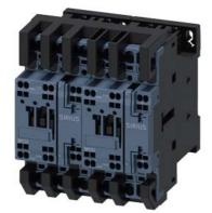
reversing contactor assembly, AC-3e/AC-3, 12 A, 5.5 kW / 400 V, 3-pole, 110 V AC, 50 Hz / 120 V, 60 Hz, spring-loaded terminal, electrical and mechanical interlock, auxiliary contacts:  $2 \times 1$  NO
