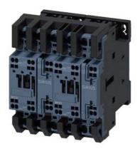
reversing contactor assembly, AC-3e/AC-3, 12 A, 5.5 kW / 400 V, 3-pole, 110 V AC, 50/60 Hz, spring-loaded terminal, electrical and mechanical interlock, auxiliary contacts:  $2\times1$  NO
