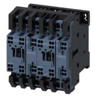
reversing contactor assembly, AC-3e/AC-3, 12 A, 5.5 kW / 400 V, 3-pole, 24 V AC, 50/60 Hz, spring-loaded terminal, electrical and mechanical interlock, auxiliary contacts: 2 x 1 NO
