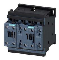
reversing contactor assembly, AC-3e/AC-3, 12 A, 5.5 kW / 400 V, 3-pole, 220 V AC, 50 Hz / 240 V, 60 Hz, screw terminal, electrical and mechanical interlock, auxiliary contacts: 2 x 1 NO
