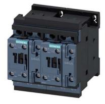
reversing contactor assembly, AC-3e/AC-3, 12 A, 5.5 kW / 400 V, 3-pole, 24 V AC, 50/60 Hz, screw terminal, electrical and mechanical interlock, auxiliary contacts: 2 x 1 NO
