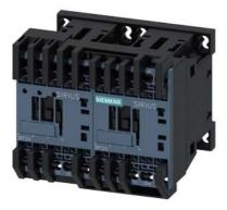
reversing contactor assembly, AC-3e/AC-3, 9 A, 4 kW / 400 V, 3-pole, 24 V DC, spring-loaded terminal, electrical and mechanical interlock, with voltage tap for  $3\rm RA27$
