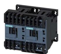
reversing contactor assembly, AC-3e/AC-3, 9 A, 4 kW / 400 V, 3-pole, 24 V DC, with integrated diode, spring-loaded terminal, electrical and mechanical interlock
