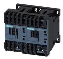
reversing contactor assembly, AC-3e/AC-3, 9 A, 4 kW / 400 V, 3-pole, 48 V AC, 50/60 Hz, spring-loaded terminal, electrical and mechanical interlock
